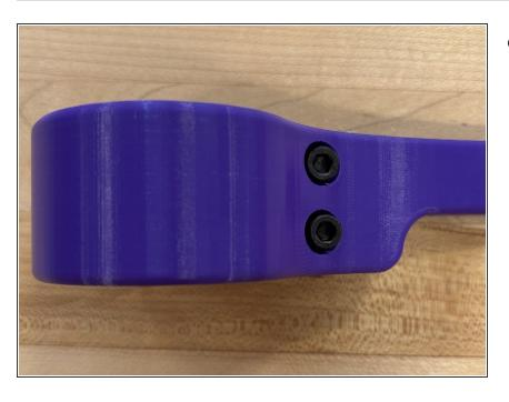
Insert the 2 M5x30mm bolts through the circular holes in the handle
